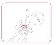
Adjust the rearview mirrors to an appropriate position and then tighten nuts on the rearview mirror with a spanner. Properly set the dust cover. Install the right rearview mirror in the same way.
