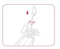
Take out the rearview mirrors and check them carefully. Install the left rearview mirror into the mounting hole on the left brake lever and turn it clockwise. The bolt shall be screwed in for more than 15 mm.
