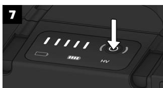
Turn off the battery by holding the on/off button for 3 seconds. All LEDs on the battery will turn off after this.
