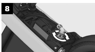
Then reconnect the battery pack to the Brekr. Tighten the bayonet fitting by turning it clockwise and make sure it clicks into place.
