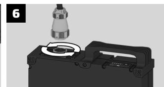
When the battery is sufficiently charged, unscrew the bayonet connector on the battery.
